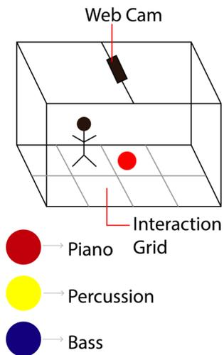
Figure 2: A diagram of the *Sound Happening* installation. Participants interact with balls while standing underneath a webcam that tracks the motion of the balls. Participants stand on an invisible grid, where movement from one section of the grid to another causes different sounds to play. Each grid section maps to a different tone and each ball maps to a different instrument.
